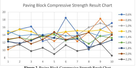
Figure 2. Paving Block Compressive Strength Result Chart Source: Compression Test Acumulation
