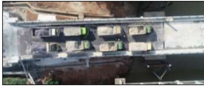
Figure 15. Documentation of the 64% UDL loading
