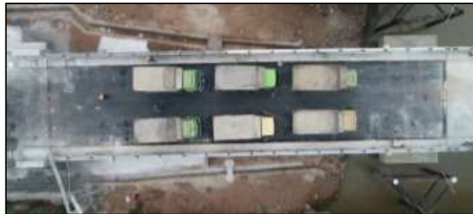
Figure 13. Documentation of the 48% UDL loading
