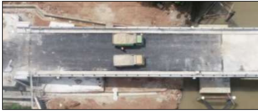
Figure 9. Documentation of the 16% UDL loading
