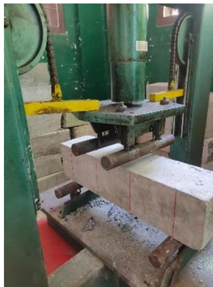
Figure 2. Hydraulic Centre-point Loading Arrangement for The Plain-concrete Beam Test
