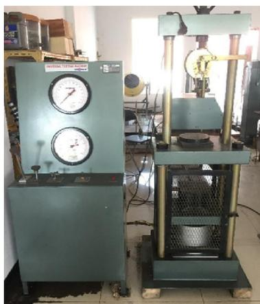
**Gambar 3. Universal testing machine tatonas type TC-325**
