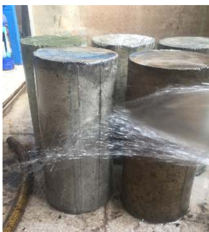
Gambar 4. Beton perawatan disiram
