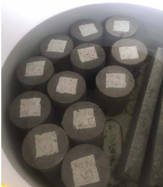
Gambar 3. Beton perawatan direndam
