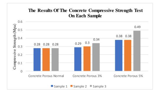
*Source: Research Data* **Figure 4.** Graph of the Compressive Strength of Porous Concrete
