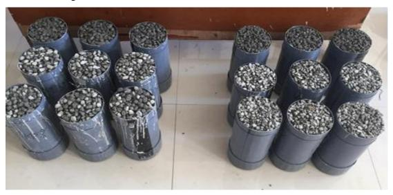
Source: Research Documentation Figure 1. Porous Concrete Specimen
