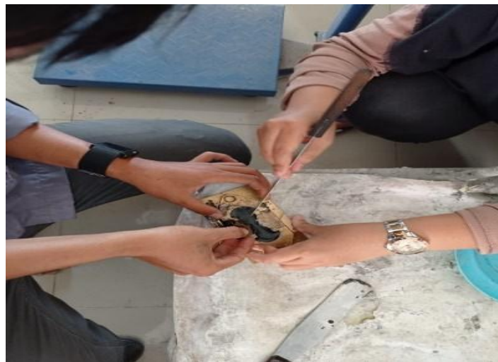
Figure 9. Asphalt Molding Process In Brass Mold
