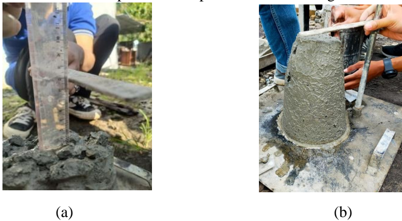
Source: Practical documentation (2022). Figure 5. Slump Test (a) Normal Concrete, (b) RCA Aggregate Concrete.
