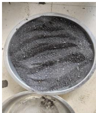
Figure 2. Fine Aggregate (Natural Sand).
