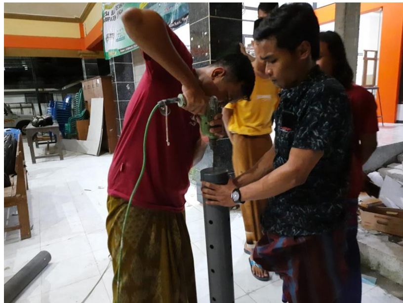
Figure 2. Production of biopores using a drill
