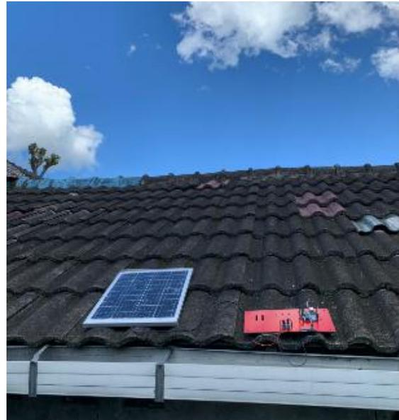
**Gambar 11. Prototype Monitoring Panel Surya berbasis IOT**
