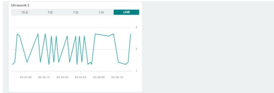
Gambar 10. Hasil monitoring ketinggian air sensor 3
