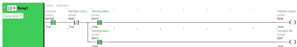
Gambar 11. Rung 1 ketika Machine Is Busy Mendeteksi Barang
