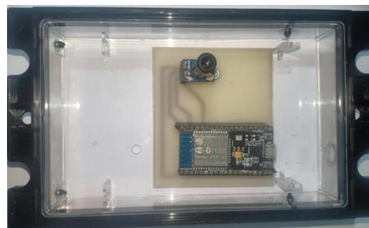
Gambar 25. Alat Monitoring Suhu Klem 20 kV
